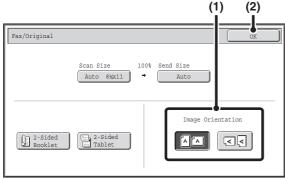
Specify the orientation in which the original is placed.
