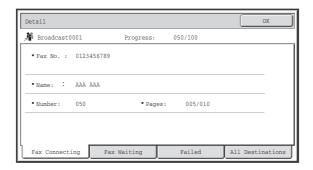
The job name and progress (number of completed destinations / total destinations) appear at the top of the screen. Touch a tab to display the information that appears on that tab. The following information appears on each tab.
