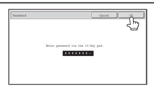
Enter a password (5 to 8 digits) with the numeric keys and touch the [OK] key.
