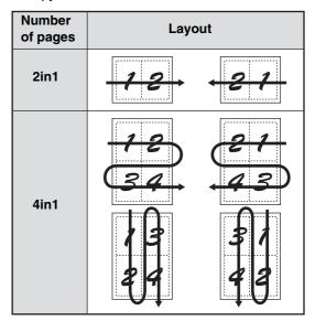
The arrows in the above diagram indicate how the images are arranged.
