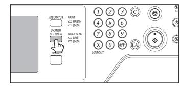
Make sure that the machine is in the standby state and then press the [SYSTEM SETTINGS] key on the operation panel.
