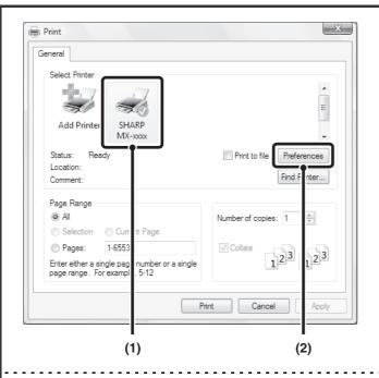
Open the printer driver properties window from the print window of the software application.
