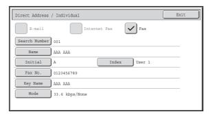
The information stored in the global address book is automatically entered. (The settings can be changed if needed. For detailed information on each item, see "Address Control" (page 7-16) in "7. SYSTEM SETTINGS".) However, configure the items below manually. To complete the storing procedure, touch the [Exit] key.
