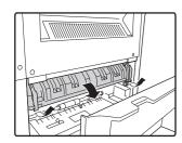
Push down the projections on the fusing area paper guide to open the fusing area paper guide, and then carefully remove the misfed paper.
