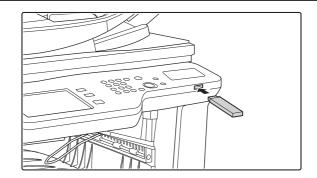
Connect the USB memory to the USB connector (Type A) on the machine.
