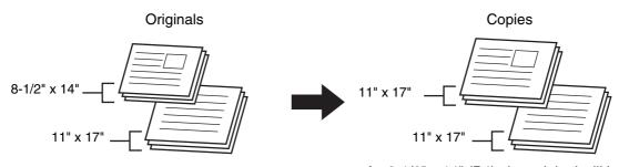
An 8-1/2"  $\times$  14" (B4) size original will be enlarged to 11"  $\times$  17" (A3) size.
