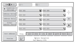
When destinations of other scan modes are stored in addition to fax destinations, an icon indicating the mode appears together with the name of the destination in each one-touch key.
