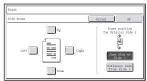
Touch the checkbox of the edge that you wish to erase and make sure that a checkmark ( ) appears.
