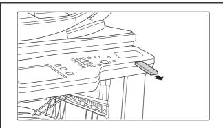
When "Sending data has been completed." appears in the touch panel, disconnect the USB memory.
