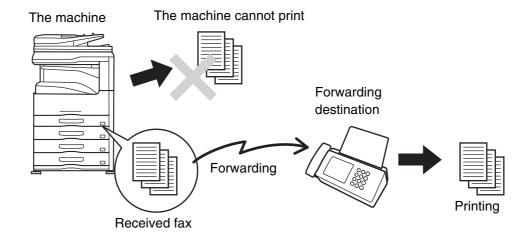
Forwarding of received faxes is executed in the system settings of the machine. Press the [SYSTEM SETTINGS] key on the operation panel to display the system setting menu screen in the touch panel. Select [Fax Data Receive/Forward] - [Fax Settings], and then touch the key that executes received fax forwarding.
