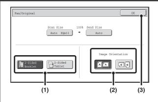
Specify the binding style of the 2-sided original (book or tablet) and the orientation in which the original is placed.
