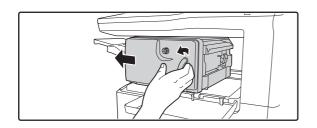
While pressing the lever over to the left, slide the finisher to the left until it stops.
