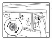
Turn roller rotating knob in the direction of the arrow to remove the misfed paper.
