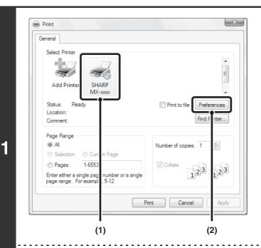
Open the printer driver properties window from the print window of the software application.
