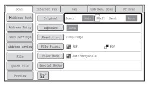
In the above screen, the scan size (the placed original) is 8-1/2" x 11" (A4) and the send size is auto. For example, if the scan size is 8-1/2" x 11" (A4) and the send size is 5-1/2" x 8-1/2" (B5), the image will be reduced before transmission.
