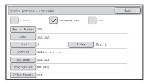
The information stored in the global address book is automatically entered. (The settings can be changed if needed. For detailed information on each item, see "Address Control" (page 7-16) in "7. SYSTEM SETTINGS".) However, configure the items below manually. To complete the storing procedure, touch the [Exit] key.
