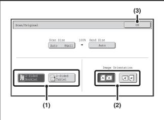
Specify the binding style of the 2-sided original (book or tablet) and the orientation in which the original is placed.
