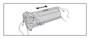
Securely hold both ends of the new toner cartridge which has been removed from its bag, and shake it horizontally 20 times.
