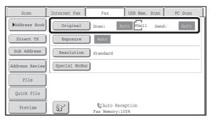
In the above screen, the scan size (the placed original) is 8-1/2" x 11" (A4) and the send size is auto. If, for example, the scan size were 8-1/2" x 11" (A4) and the send size were 5-1/2" x 8-1/2" (B5), the image would be reduced before transmission.
