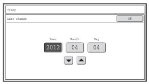
As an alternative to touching the keys, you can also directly touch the numeric value display key and change the value with the numeric keys.
