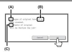
When scanning is completed, check the number of original sheets and the number of sheets to be sent, and touch [OK].
