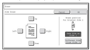
Touch the checkbox of the edge that you wish to erase and make sure that a checkmark ( $\checkmark$ ) appears.
